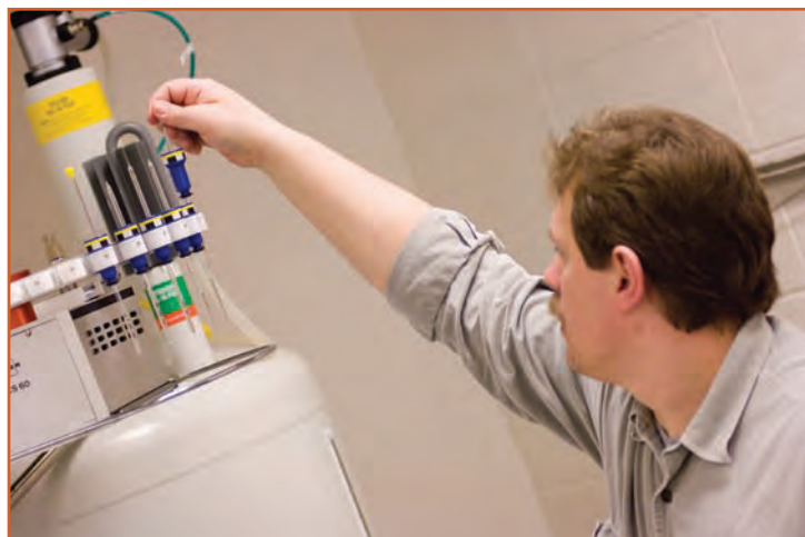
Richard Fitch, assistant professor of chemistry, loads a chemical sample into the sample changer of a new 400 MHz nuclear magnetic resource spectrometer.
